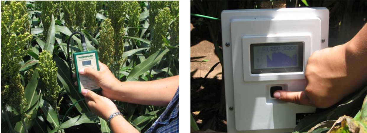
Figure 1-2A–B. Soil moisture data collection from one field with a manual data logger (left) and another field’s data collection with an electronic data logger (right).
